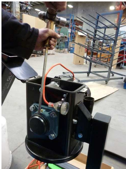
3. Carefully wedge black cap off bearing.
