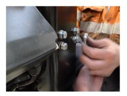
8. Loosely fit back two bolts 2-3 threads
