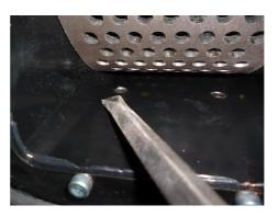
2. If set screws protruding wind the out to avoid contacting screen
