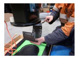
5. Locate screen so that feather edge catches in housing. With shoulder against Jack pull / spring screen so that it drops up into housing
