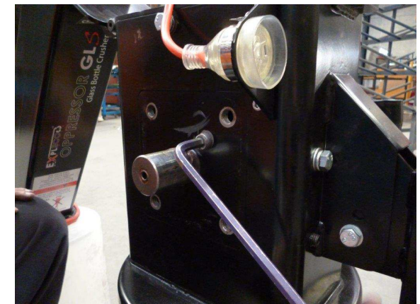
7 - Undo 16mm Alan Screw to access pin ends
