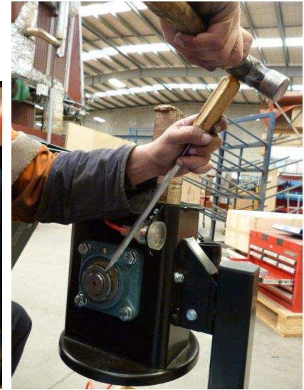
4 - Firmly hit nut to undo. Undo at least 3 thread. Approx. 6mm
