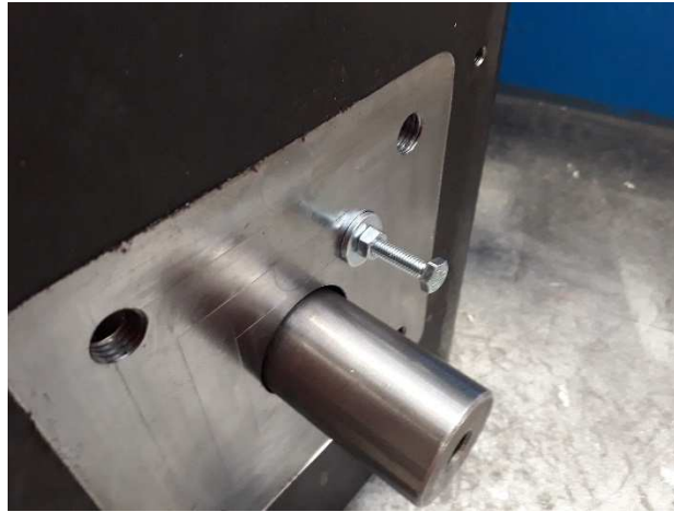
9 – Using 6mm puller (available from Expleco) work pins free and pull out by hand.
