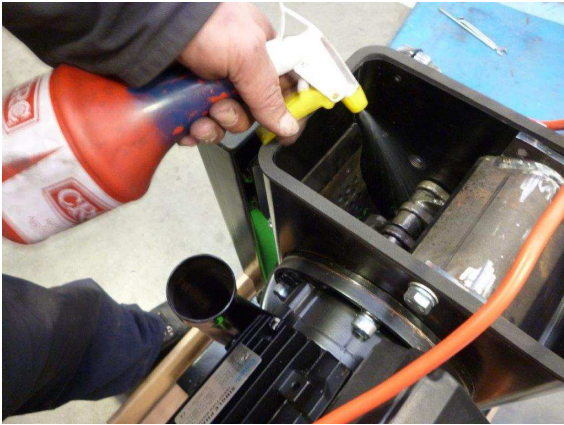
1 - Liberally spray hammer pins with penetrant. Spray daily for 2-3 days before hammer Replacement.
