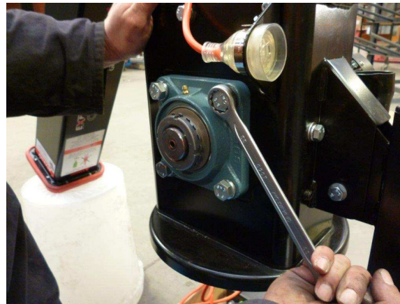
6 - Undo bearing bolts and remove bearing
