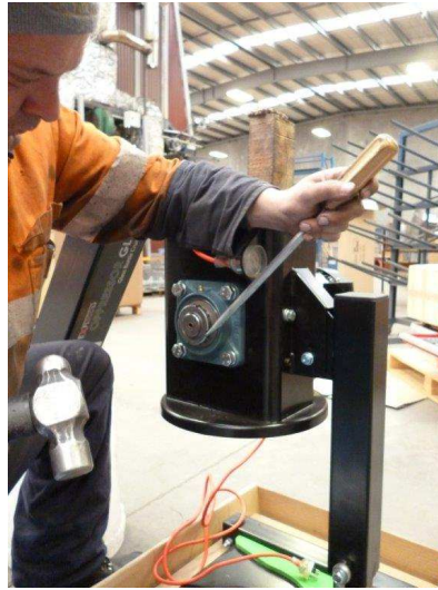
15 – Re-install 16mm Alan Key at pin ends. Make sure it is flush inside Housing. Re-fit bearing and locking Tab and nut. After nut has begun Wedge it ot to pull taper lock out. Wind nut finger tight and then firmly Tap with large screw driver and hammer Until nut is solid hit tight and a tab aligns To enable folding back into place.
