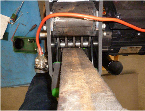
14 – Fit Block of wood to lock rotation
