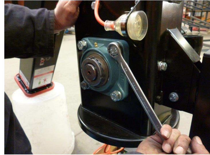
16 – Tighten 4 bearing bolts firmly and then back off ¼ turn.
