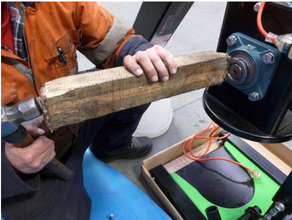
5 - Firmly hit nut to release taperlok. Remove Nut
