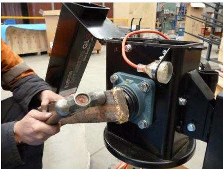
17 - - Finally replace the bearing cap carefully tapping with a block of wood or rubber hammer.
