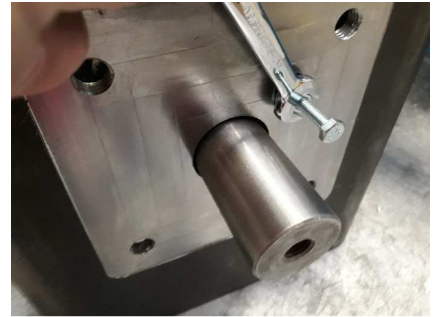
10 - or use Spanner to wind out using puller nut.
