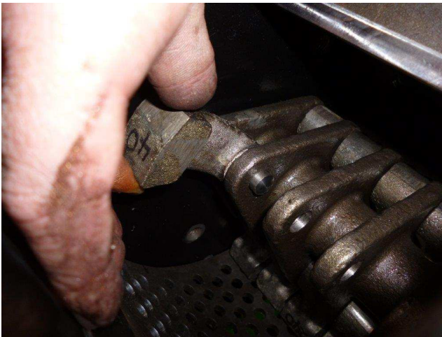
11 – Replace hammers . As per orientation
